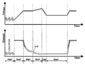
Reference charging time (hours) to 85 % capacity. Time varies with different batteries and conditions. 25Ah: 5h 75Ah: 9h 100Ah: 16h 150Ah: 24h
