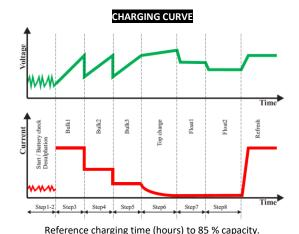
Time varies with different batteries and conditions. 25Ah: 5h 75Ah: 10h 100Ah: 18h 150Ah: 26h Note: If left connected, it is programmed to restart from
